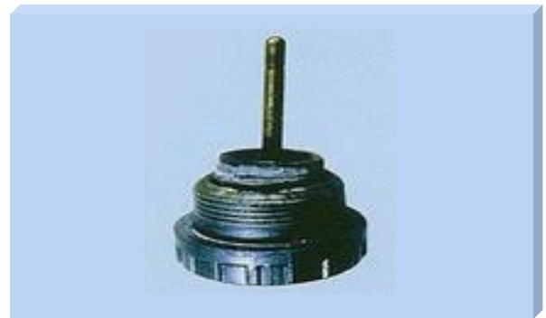
Rust of valve parts
