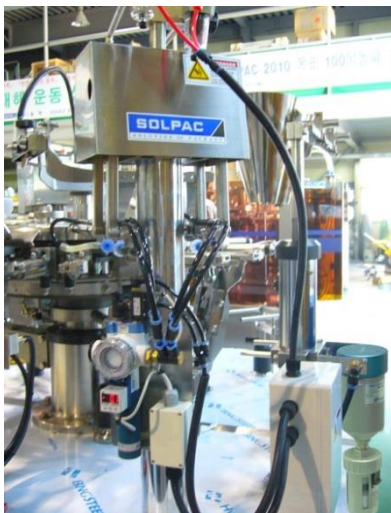
▲ Vacuum pump and pneumatic actuator of packaging machine
